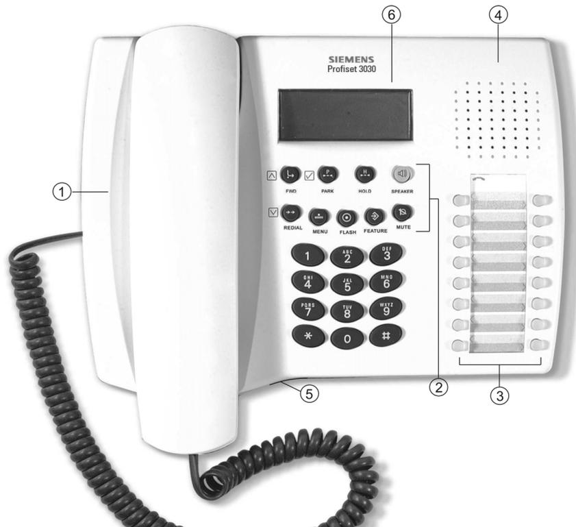
Figure 5-1 Profiset 3030 System Telephone Layout
